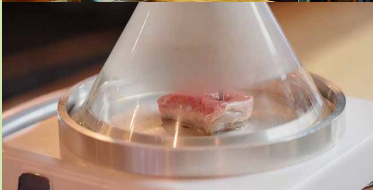
Top: Dr Santanu Deb-Choudhury with chef Dale Bowie, of Sheppard restaurant in Wellington, analysing data captured by DART-MS; Bottom: Volatiles are monitored in real time during the cooking of a piece of steak.
