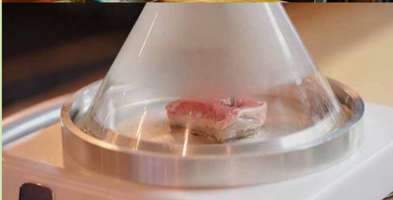
Top: Dr Santanu Deb-Choudhury with chef Dale Bowie, of Sheppard restaurant in Wellington, analysing data captured by DART-MS; Bottom: Volatiles are monitored in real time during the cooking of a piece of steak.
