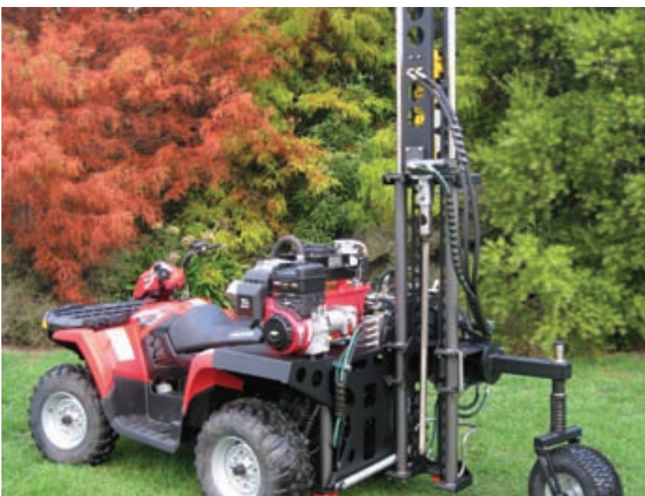
The purpose built ATV mounted hydraulic soil sampler built by the Lincoln-based Engineering team.
